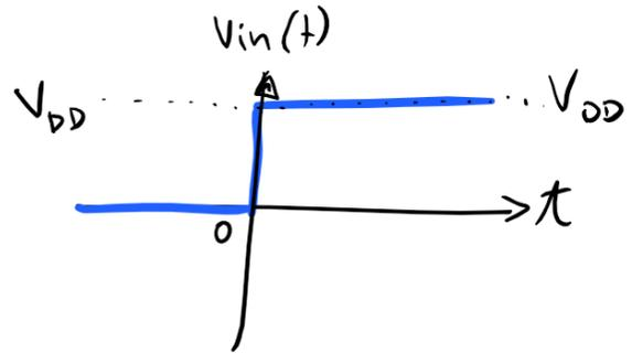
If  $v_{in}(t)$  is as plotted above, please provide a differential equation in  $v_{out}(t)$ . (5 points)
