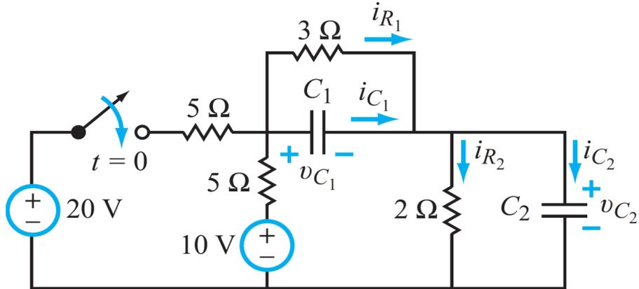
a) What is  $i_{C_1}(t=0)$ ? Show your work!**Solution:**b) What is  $i_{R_1}(t=0)$ ? Show your work!**Solution:**c) What is  $v_{C_1}(t=\infty)$ ? Show your work!**Solution:**
