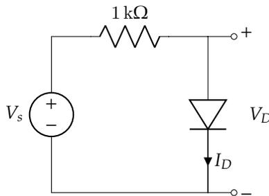
Here  $I_s$  is the saturation current and  $V_{TH}$  is the thermal voltage both of which depend on the device physics. To obtain experimental data, Taejin applies voltages  $V_s$  and measures voltages and currents  $V_D$  and  $I_D$  across the mystery device. **Set up and solve a least-squares problem in the Jupyter Notebook to estimate  $I_s$  and  $V_{TH}$ .**
