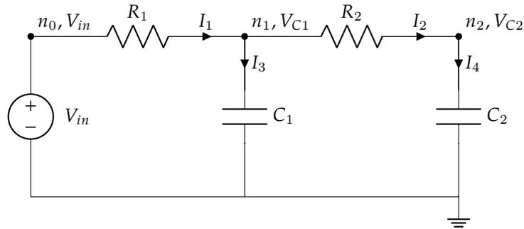
Figure 4: Two dimensional system: a circuit with two capacitors, like the one in lecture.
