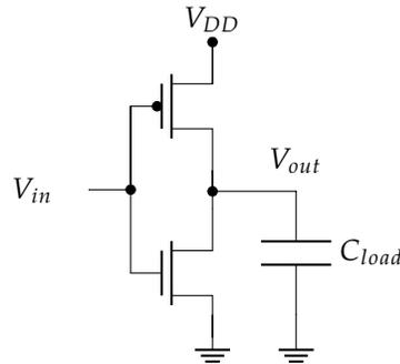
Figure 1: CMOS Inverter driving a capacitive load.
