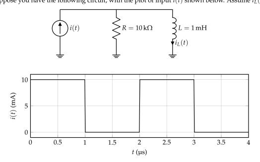
(a) (5 pts.) Find the differential equation for *i*<sub>L</sub>(*t*) in terms of *R*, *L*, and *i*(*t*).Solution: To start out, let's write out the KCL equation for the circuit.
