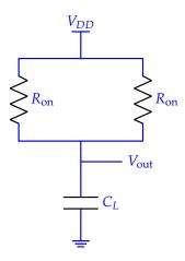
This time, there are two resistors connected to the output node in parallel, so the time constant is  $\tau_2 = \frac{1}{2}R_{on}C_L$ .
