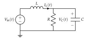
(a) (6 pts.) **Derive a set of differential equations, one for**  $I_L(t)$  **and another for**  $V_C(t)$ **. Solution:** We begin by using our circuit analysis methods. Using KVL and replacing the inductor voltage, we obtain:
