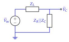
where  $Z_R ||Z_C = \frac{Z_R Z_C}{Z_R + Z_C} = \frac{(R)(\frac{1}{j\omega C})}{R + \frac{1}{j\omega C}} = \frac{R}{1 + j\omega RC}$  and  $Z_L = j\omega L$ .
