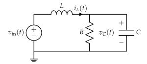
(a) (8 pts.) Find the differential equation for  $v_C(t)$  in the following form (where *a*, *b*, and *c* are constants that depend on *R*, *L*, and *C*):
