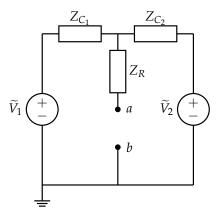
Here,  $Z_R = R$ ,  $Z_{C_1} = \frac{1}{j\omega C_1}$ , and  $Z_{C_2} = \frac{1}{j\omega C_2}$ . You may assume that the value of  $\omega$  is fixed (i.e., the time domain representations of  $\tilde{V}_1$  and  $\tilde{V}_2$  both have the same angular frequency). Find the Thevenin equivalent impedance between ports *a* and *b*.
