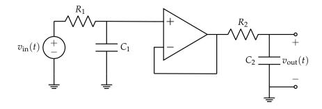
Suppose  $v_{in}(t)$  is some sinusoidal input, and the input and output voltage phasors are denoted  $\tilde{V}_{in}$  and  $\tilde{V}_{out}$  respectively. Write the transfer function for this circuit.
