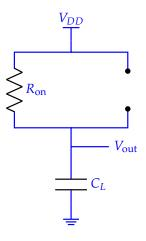
There is just one resistor  $R_{on}$  and one capacitor  $C_L$  connected to the output node so we can say that the time constant is  $\tau_1 = R_{on}C_L$  (you could also write the differential equation for this). For Scenario 2, we know that transistor M1 and M2 are both on. Thus, the equivalent circuit will look like this:
