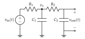
Again, assume  $v_{in}(t)$  is sinusoidal, and the phasor representations of the input and output voltages are  $\tilde{V}_{in}$  and  $\tilde{V}_{out}$  respectively. Find  $\tilde{V}_x$ , the phasor representation for  $v_x$  in the circuit above, in terms of  $\tilde{V}_{in}$ .
