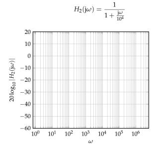
**Solution:** Again, we have a low-pass filter but with cutoff frequency  $\omega_c = 10^4$ :
