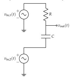
(a) (7 pts.) Find the **transfer function**  $H_1(j\omega_1) = \frac{\tilde{V}_{\text{out},1}}{\tilde{V}_{\text{in},1}}$  that describes the contribution of  $v_{\text{in},1}(t)$  to the output voltage.
