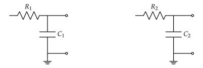
We know from lecture that these circuits represent low-pass filters. In this problem, we will demonstrate the loading effect and hence motivate the need for a unity gain buffer when cascading filters.
