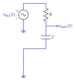
The transfer function in this case is that of RC low pass filter:
