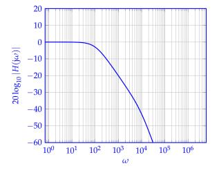
This is clearly not the same as the Bode plot which we obtained when we cascaded the two filters with a unity gain buffer.
