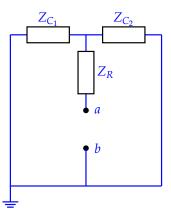
Combining  $Z_{C_1} \parallel Z_{C_2}$  into a single element, we see that  $Z_{TH} = (Z_{C_1} \parallel Z_{C_2}) + Z_R = R - \frac{j}{\omega(C_1 + C_2)}$ .
