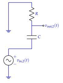
The transfer function in this case is that of CR high pass filter:
