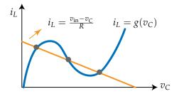
Let  $v_{in}^*$  be a constant input voltage and let  $(v_C^*, i_L^*)$  denote one of the resulting equilibrium states, that is one of the intersections of the two curves above. Since the right-hand side of (6) has the form
