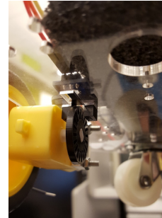
(b) Bottom view of encoders
