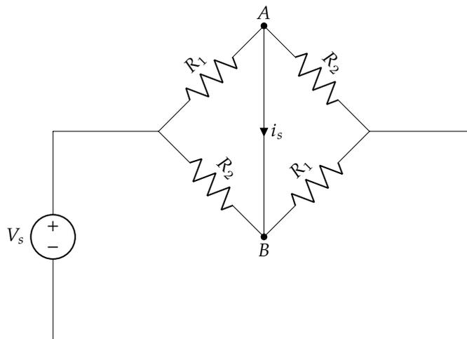
Figure 2: Modified Wheatstone bridge circuit.
