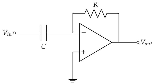
Figure 4: Operational Amplifier with RC elements.
