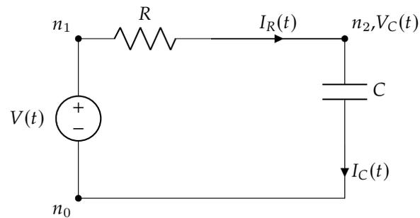
Figure 1: Example Circuit
