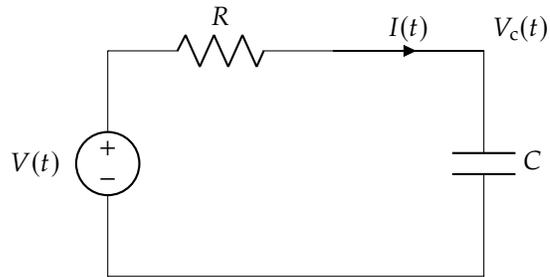
Figure 4: Example Circuit
